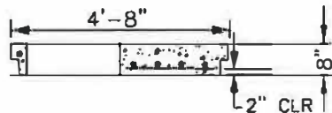
SLAB FOR 4'-0" I.D. MANHOLE
