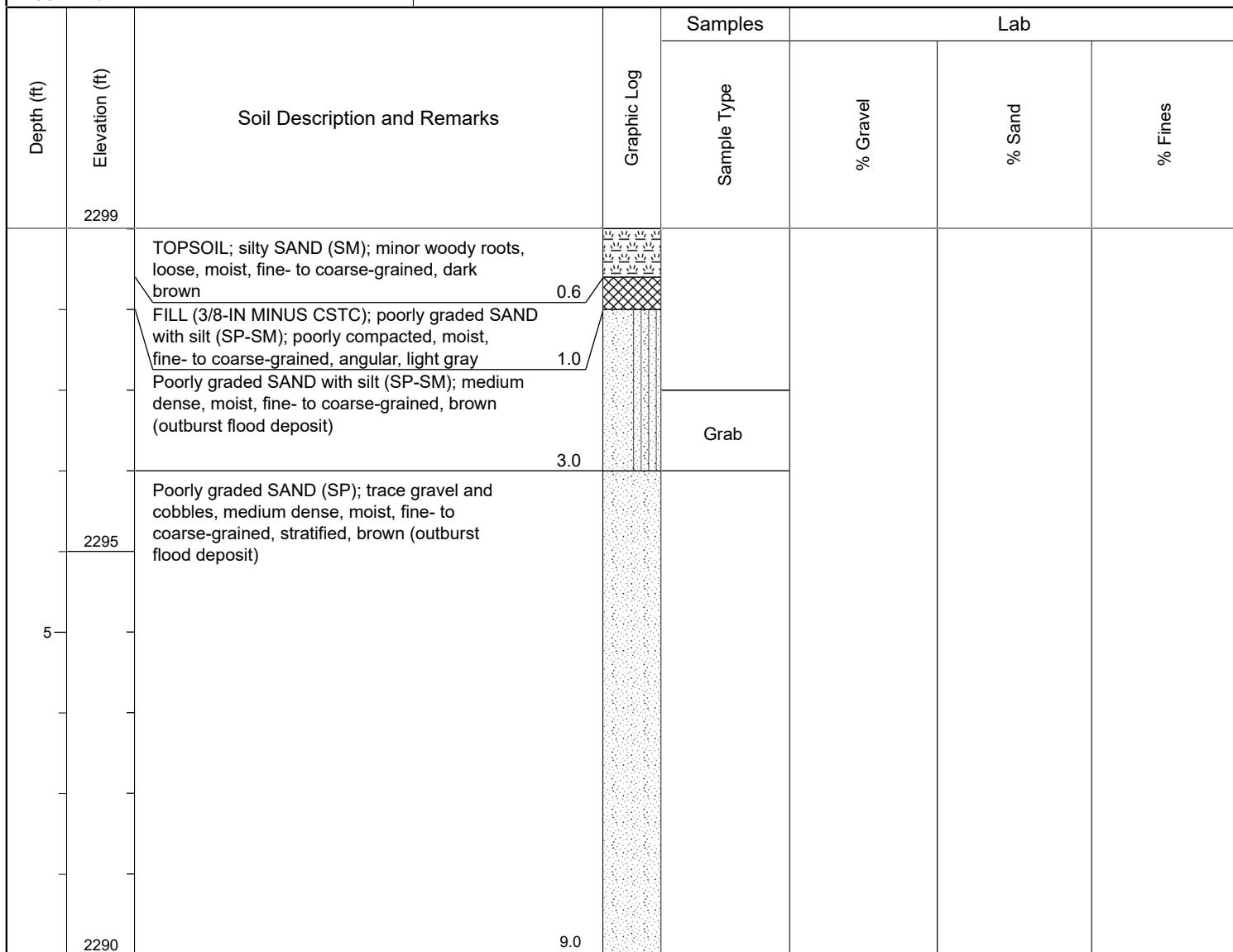
Test pit terminated at 9 feet due to caving.
