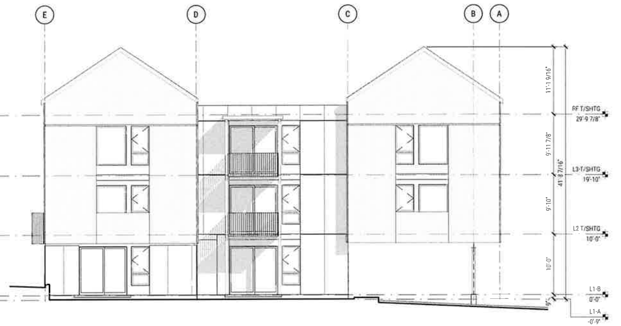
02 EXTERIOR BUILDING ELEVATION - EAST SCALE 1/8" = 1'-0"
