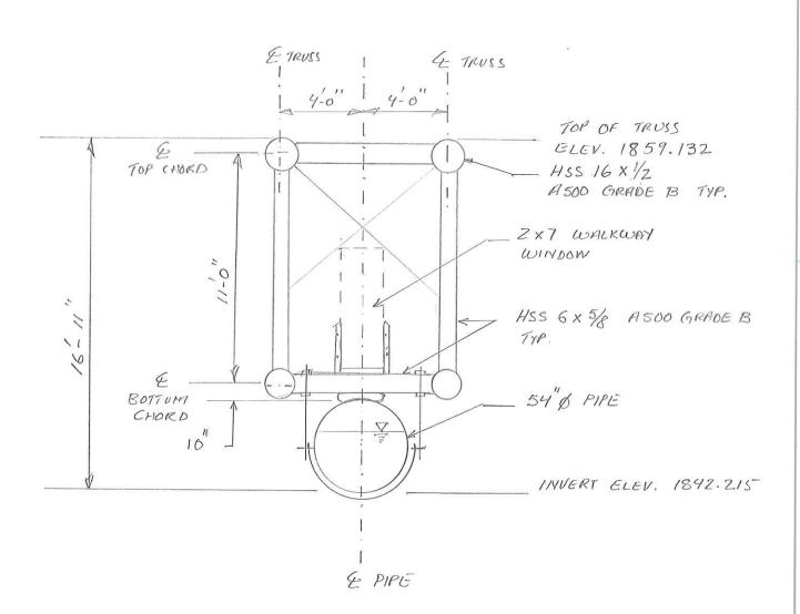
PROJECT POST ST. BRIDGE 7SEL CONT SUBJECT PIPELINE TRUSS TEMP BRIDGE PAGE ASIL DATE 7/4/2015 CALCULATIONS BY \_\_\_\_ CHECKED BY\_ DATE ALTERNATIVE 2 - PILE ROCK SOCKET TYP. 45-0" CANTILEVER 11-0" STRUCTURE DEPTH 54 % PIPE 54" SEWER TRUSS BOTTOMY CHORD BRIDGE LAYOUT BEARING FRAME (STEEL) 250-0 ELEV. 1833.2 - 100 YR FLOOD 16-0" TYP. NO ABUTMENTS NEEDED 17 14 E BRIDGE & I PIPE SECTION A-A 4 CANTILGVER 45-0"
