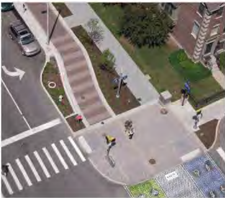
Figure 42. Tighter curb radii slows traffic and increases safety
