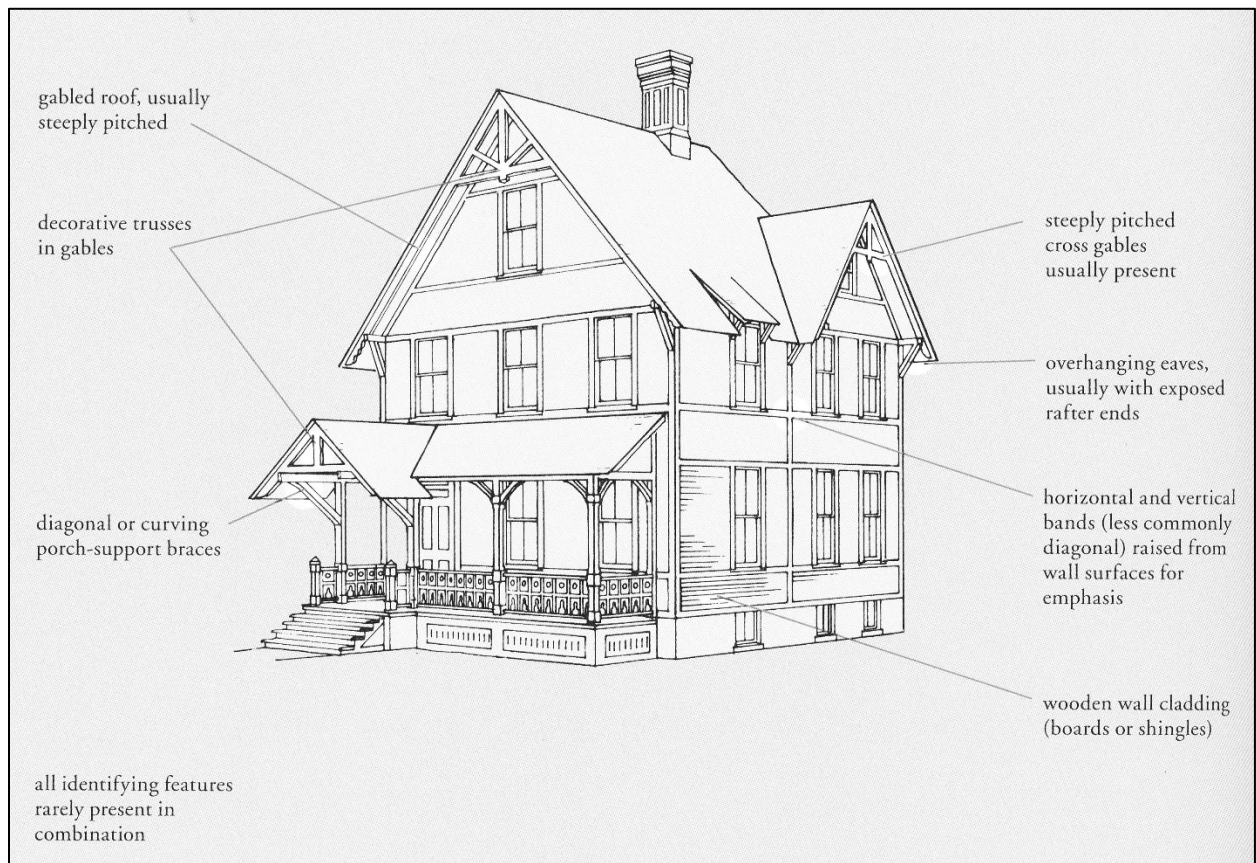
Figure 16: Diagram of a Stick Style house
