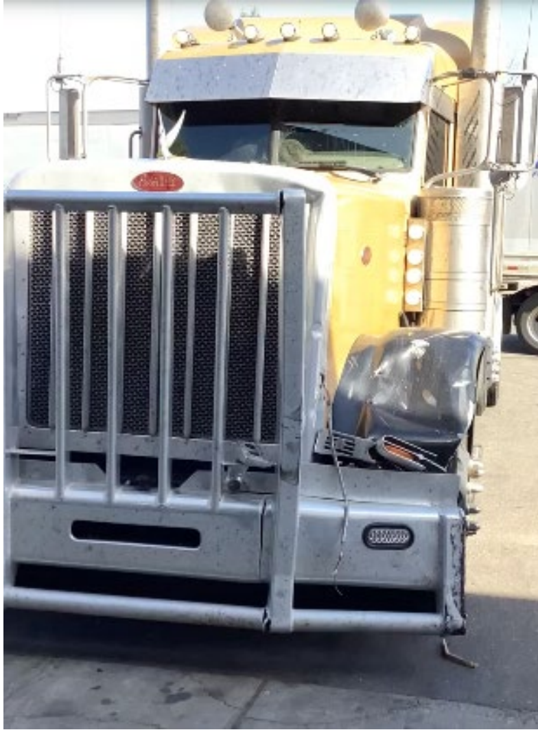
Deer strike. Hood as repaired, crown and bumper replaced.
