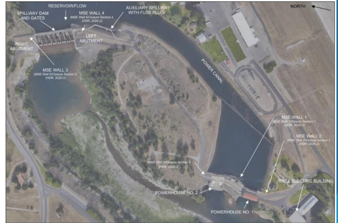
Figure 1-1. Upriver Hydroelectric Project Site Layout
