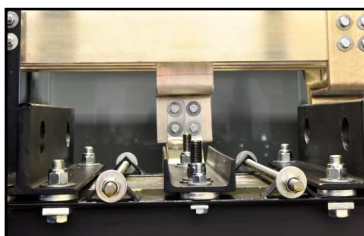
Lifting eyes for core & coil assembly
