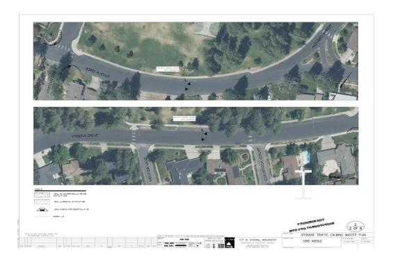
In addition to the speed humps above there are curb extensions proposed. I can see some benefit to this as it narrows the intersection and gives pedestrians an island of safety. However we would not be opposed to an adaptive solution for this feature as I am less convinced of the need here. An adaptive solution would save money and allow us to test drive the need for the bump outs.
