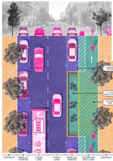
FIGURE 11 Cross-section of the long-term vision for Sprague and 1st Avenues prioritizing active transportation and public space. The location of protected bike lane will be impacted by the transit stops.
