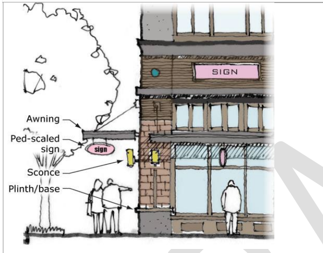
((Figure 17C.123.060-A: Illustration of building base, pedestrian scale signs and other building elements described in the FBC.))
