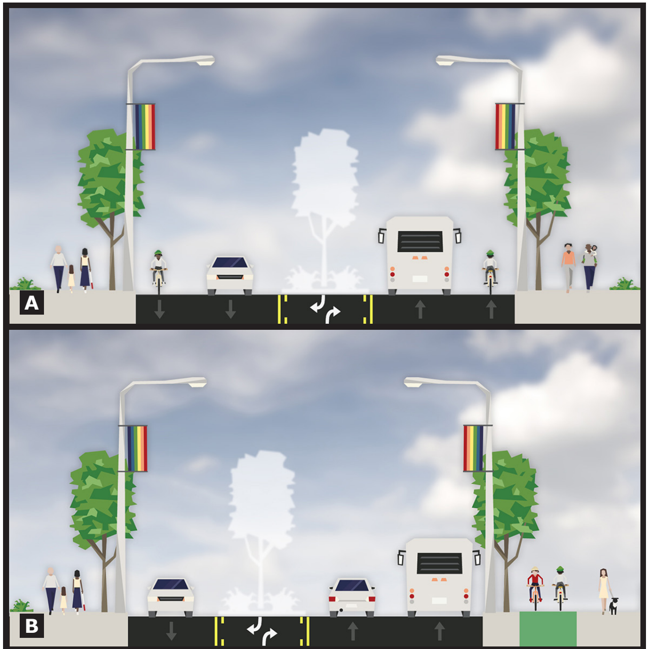
Figure 2.03 – Two options for FGW were examined for this plan: A preferred three-lane configuration ("A") and a four-lane version ("B"). Both sections depict center turn lanes, with landscaped medians "ghosted" in to indicate alternating conditions. Reconfiguring FGW is seen as a critical step in achieving many key objectives, including a more gracious, welcoming environment for pedestrians and cyclists, smoother traffic flow, and improved safety for all. (Image, Studio Cascade, Inc.)
