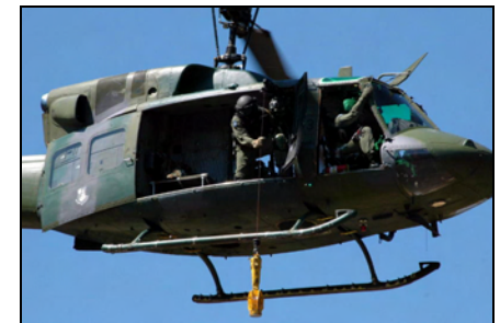
36 RQF UH-1 with a jungle penetrator extraction device
