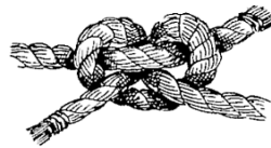
FIG. 14.—Slipped square knot.
