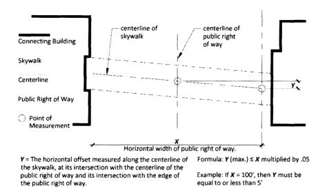
2. The vertical slope of the skywalk structure should not exceed one percent of the width between the connecting buildings' contact points. (P)
