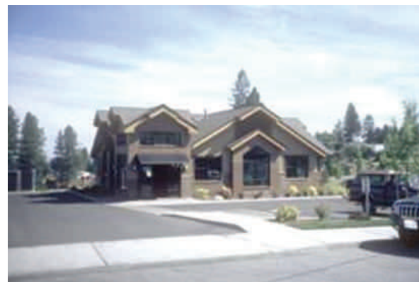
6 inch vertical curb defines pedestrian connection
