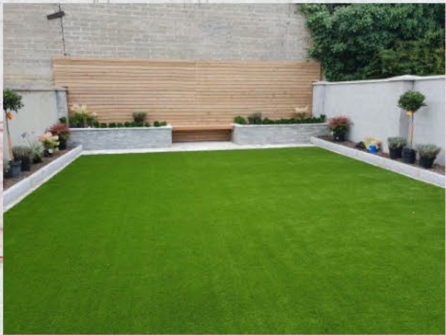
SYNTHETIC TURF, LOW MAINT, GOOD SHOCK ATTENUATION, PERVIOUS.
