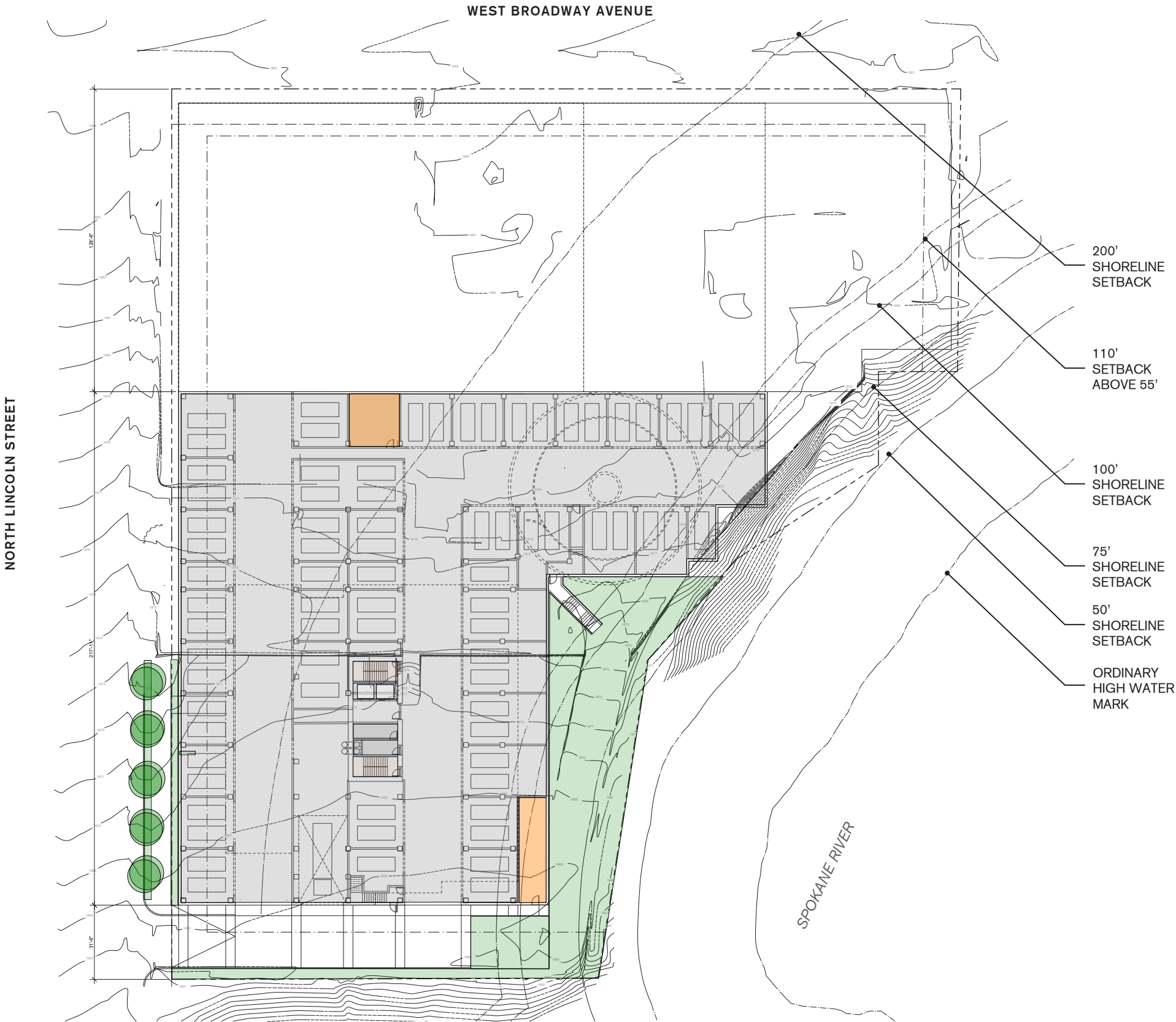
LEVEL P1 FLOOR PLAN SCALE: 1" = 50'-0"
