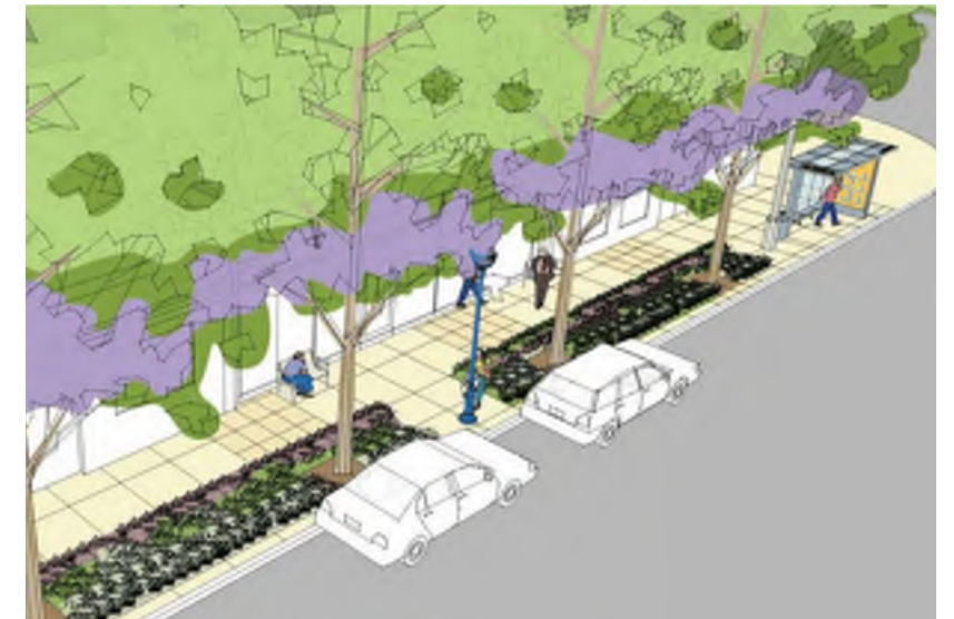
Curbside planting strips should be used in busy traffic areas to separate vehicle traffic from the pedestrian sidewalks and plazas.
