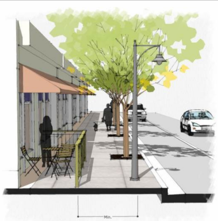
((Figure 17C.123.050-F: Temporary sidewalk encroachments are allowed in the Planting Zone, or in the Clear Pedestrian Zone as per Table 17C.123.050-4.))
