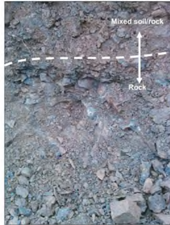
Photograph 6 – View of TP-6 sidewall showing mixed soil and rock overlying fractured basalt rock.
