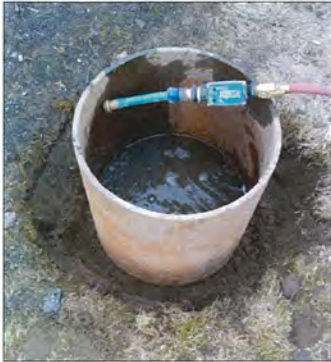
Photograph 1 – View of single-ring infiltration test performed in TP-4 (Pond C).
