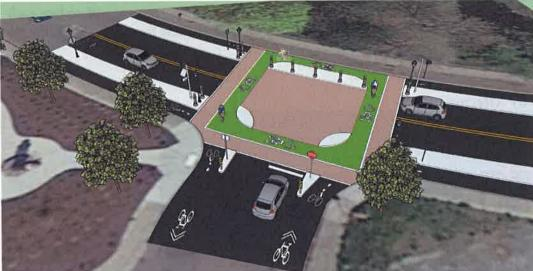
Figure D10 - A potential future design for the N Belt St, N Pettet Dr, and W Maxwell Ave intersection, which borrows themes from protected intersections to create a safer, seamless transition between the Chestnut Corridor Greenway and the Pettet/Maxwell bike lanes.
