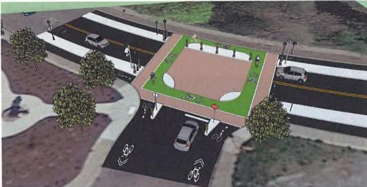
Figure D10 - A potential future design for the N Belt St, N Pettet Dr, and W Maxwell Ave intersection, which borrows themes from protected intersections to create a safer, seamless transition between the Chestnut Corridor Greenway and the Pettet/Maxwell bike lanes.
